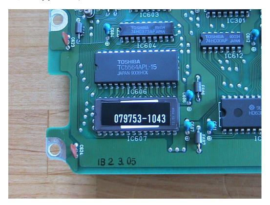
Once you've located the chip, flip the board over and desolder it from the board. Take your time.
