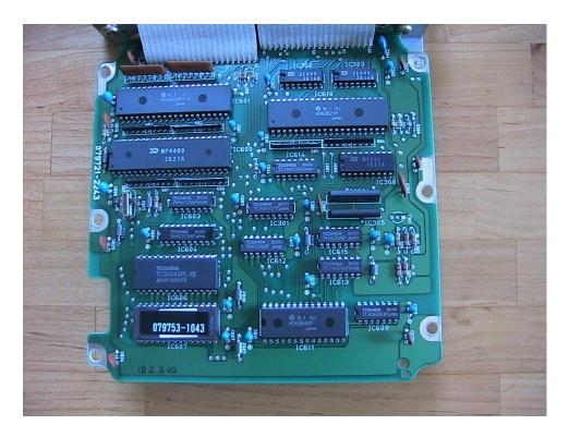
We need to remove IC607 (the chip with the stick on label at the bottom left of the above picture, closeup pic below). The board will also be silk screened with IC607.
